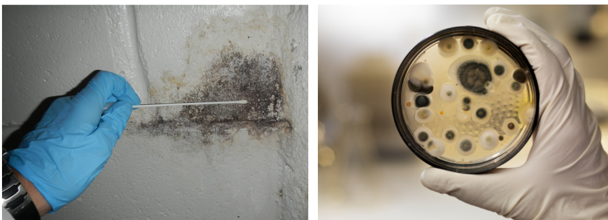
Picture 7. Microbial samples are collected from damaged surfaces and analyzed in a laboratory.
